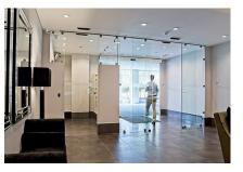
As part of the main entry lobby refurbishment to the 442 St Kilda Road apartment building, record Automatic Doors supplied and installed three STA 20 automatic sliding doors. Two of the operators were mounted in the ceiling space with record combination sensors flush mounted within the ceiling finishes.
